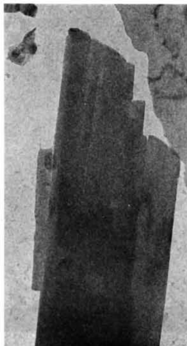
Fig. 7. Bright-field image of lath n -hexatriacontane crystals epitaxially grown in naphthalene. Calibration of image rotation to diffraction pattern (see Fig. 8) shows that molecular long-chain axes are normal to lath length.
